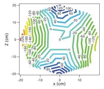
**Fig. 4.**  $B_0$  field map for the x–z plane, obtained after optimization of passive shim placement. Contours indicate deviation of  $^1$ H NMR frequency in Hz from the zero-center frequency of 210 kHz. Across a human lung of width  $\sim$ 25 cm,  $v_0 \sim \pm 80$  Hz, which implies the  $B_0$  homogeneity  $\Delta B_0 \sim \pm 0.02$ G or about 350 ppm.
