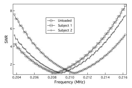
Fig. 8. Measured SWR as a function of frequency for the human chest coil unloaded as well as loaded by two different human subjects weighing between 60 and 80 kg.
