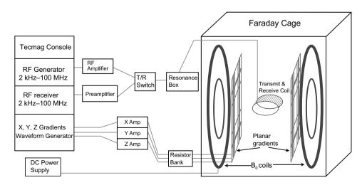
**Fig. 1.** Schematic of the open-access human MRI system. The major components include an MRI research console (left), electronics components for RF and gradient pulse generation and  $B_0$  control (center), and the  $B_0$ , gradient and  $B_1$  coils, located inside an RF-shielding Faraday cage (right). The resonance box, T/R switch and preamplifier are located inside the Faraday cage, but are drawn as shown for clarity.
