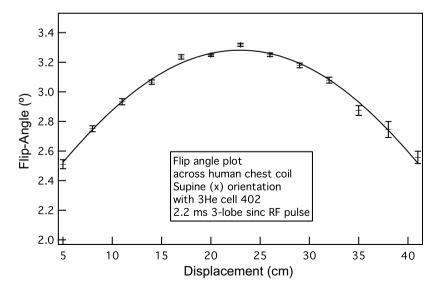
**Fig. 7.** Measured  ${}^{3}$ He flip-angle versus position along the center axis of the human chest coil oriented for supine lung imaging (i.e., along the imager's x axis). Flip-angle calibrations were performed on hyperpolarized  ${}^{3}$ He cell #402 which had a 3 cm width along the x axis. Displacement is measured from one end of the chest coil. The solid curve is a fit of the data to the function describing the  $B_1$  field created by an ideal finite solenoid.
