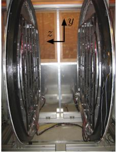
**Fig. 2.** Left: The  $B_0$  and gradient coils mounted on the aluminum flange. The arrows point to the outer and inner  $B_0$  coils. The other circular coils are the z gradient coils, while the rectangular coils are the x and y gradient coils. Right: A view of the imaging region with the imaging axes defined. The x axis points out of the page.
