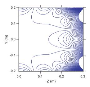
**Fig. 3.** Calculated plot of  $B_0$  homogeneity for the biplanar, four-coil arrangement. The ordinate represents the y axis of the imager and intersects the center of the magnet at zero. The abscissa represents the distance from the central y axis, along z; thus, one half of the region of interest is shown. Each contour line is a 25 ppm  $B_z$  deviation from the center  $B_0$ . The design target DSV is 0.4 m.
